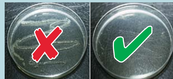
This is bacterial growth in a hold cleaned without using bleach.
